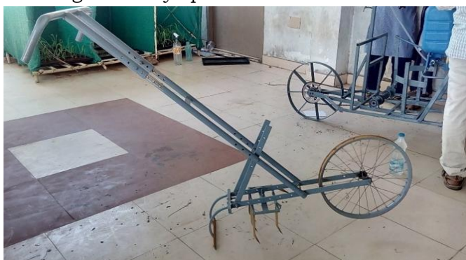
Fig - 6.Complete assembly of weeder
